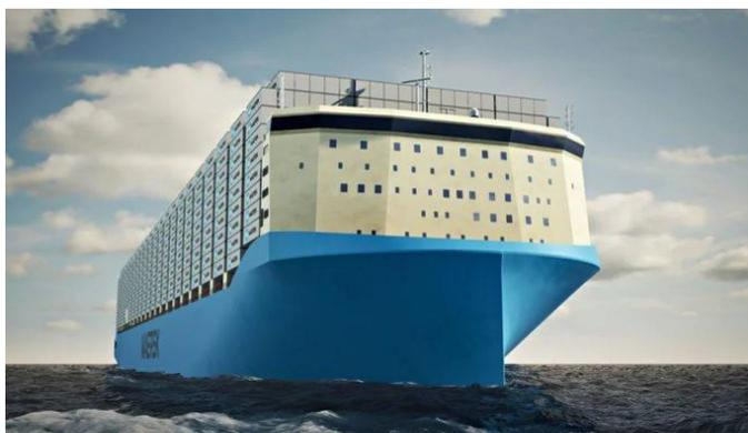
(HHI) with delivery planned for the first quarter of 2024. Most striking is the forward accommodation that Maersk says will enable greater container capacity and improved port efficiency by separating the accommodation and funnel. The funnel is also designed with a reduced footprint and will be located at the stern to maximize cargo capacity.
