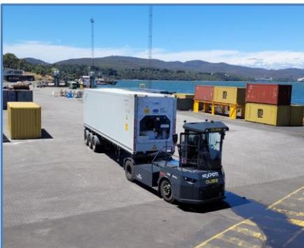
Qube is trialling a battery electric Inter Terminal Vehicle (ITV). In collaboration with Nexport and their partner Gaussin Group, Qube is trialling this cutting-edge electric ITV for their Bell Bay operations.
