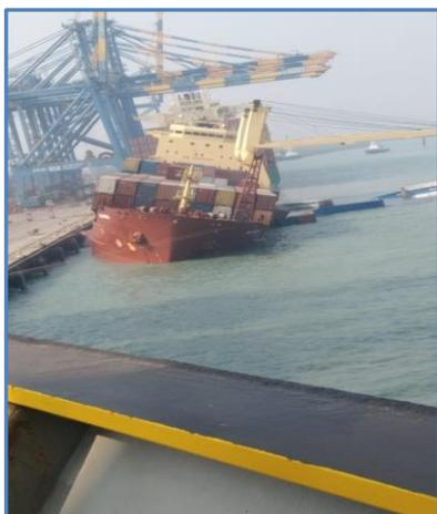
Photos from the scene suggest that before or after the accident, the vessel also listed hard to starboard, towards the wharf. There are several possible explanations for the list changing sides, including improper ballasting, sudden cargo loss, or a vessel switching between sides at the *angle of loll* (the angle of inclination of a vessel under given conditions at which this occurs is known as the angle of loll, and the vessel is said to be in a state of continuous rolling motion).
