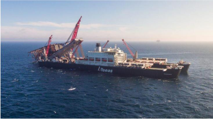
Allseas says the system makes it “fundamentally different” from conventional crane-lifting vessels and the ship’s own lifting system. The new system allows for the direct transfer of structures, eliminating the need for support barges. There is also no need to sea fasten the jacket to the beams during transit “due to the vessel’s high level of stability, significantly reducing time in the field and lowering the emissions footprint,” according to Allseas.
